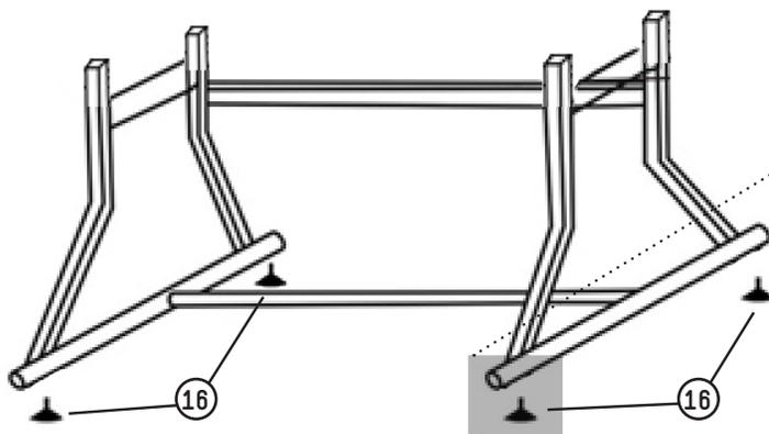
Now attach the [4] Floor Guides (Part (16)) into the base by screwing the guides into the specified holes on the bottom of the base units.
