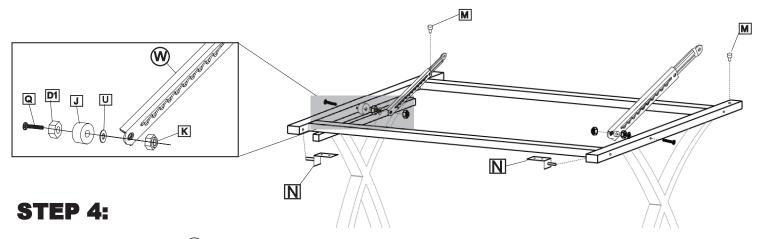
Attach Tilt Mechanism (Part (W)) to the left leg using the hole that is near the front of leg.
