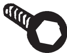
K. [4] M6 x 20 Screws Note: These screws are attached to Part [G]
